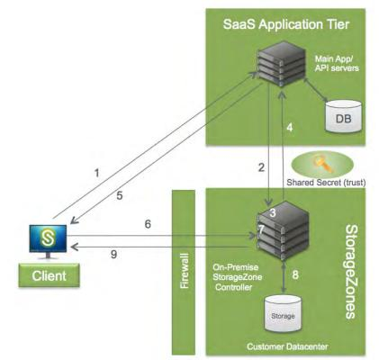
Figure 6: Preventing forged requests workflow diagram
