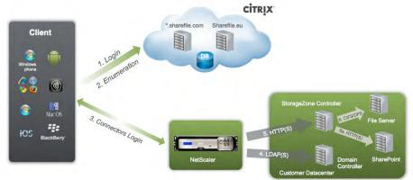
Figure 17: Securing requests for ShareFile Connector data with NetScaler
