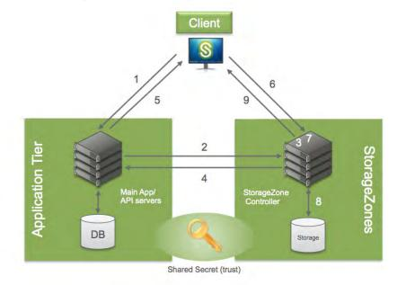
Figure 4: Preventing forged requests workflow diagram
