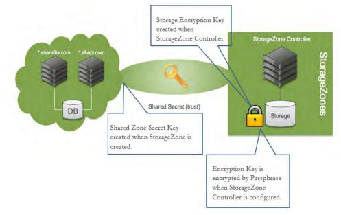
Figure 7: Security related SZ Controller configurations
