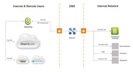
Figure 1: ShareFile components overview with applicable ports.
