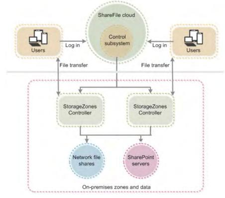
Figure 10: StorageZone Connectors component architecture
