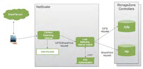
Figure 16: NetScaler configuration architectural diagram for StorageZone Connectors
