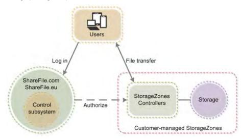
Figure 5: Customer managed on-premise StorageZones components diagram
