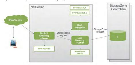
Figure 14: NetScaler configuration architectural diagram for ShareFile data
