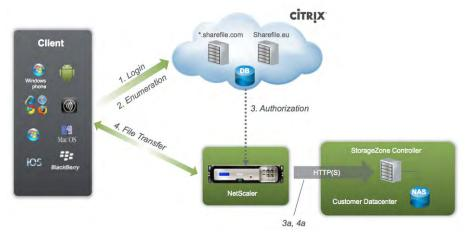
Figure 15: Securing requests for on-premise ShareFile data with NetScaler
