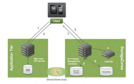
Figure 11: StorageZone Connectors workflow diagram without NetScaler
