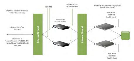
Figure 12: NetScaler components architecture for on-premise StorageZones Controllers
