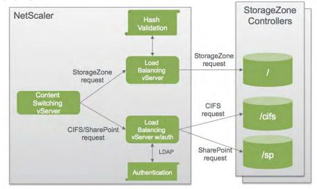
Figure 13: NetScaler configuration architectural diagram
